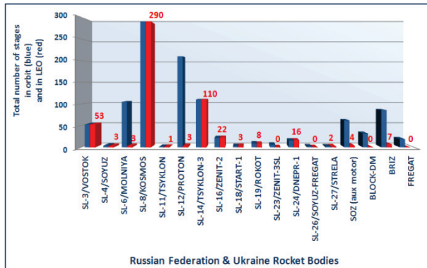
Fig. 8: Distribution among rocket types and orbital regimes of the upper stages launched by the Russian Federation and Ukraine 2 .
