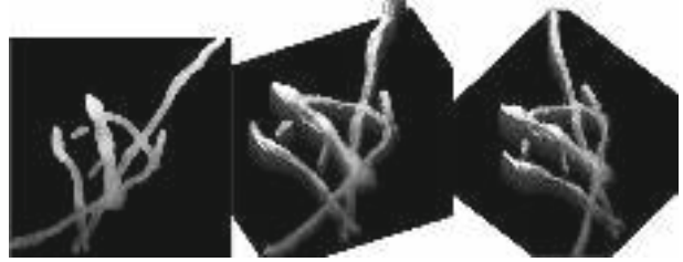
Fig. 2 Segmented microtubules as in Fig. 1, but with the application of PRIAR processing for enhancing resolution with a magnification of a factor 2. On the left : 3D representation of the tubules as input image. On the right : 3D representation of the correspondent enhanced resolution image with edges treatment as given by Eq. (11) and denoising processing
