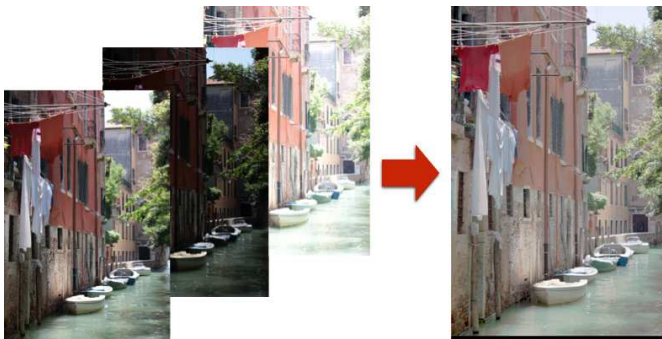
Figure 6. An example of HDR imaging from a sequence of LDR images at different exposure times
