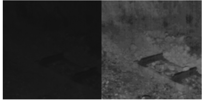
Figure 5 Night image acquired (left) and after real-time histogram adjustment (right)
