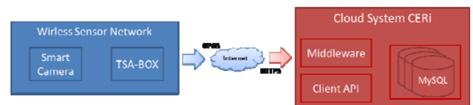
Fig. 3 – Cloud system architecture for recorded data collection.
