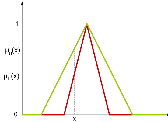
Figure 2: Interval type-2 set described by an upper (green) and a lower (red) membership function.
