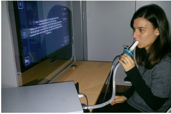
Fig. 13. The Wise Sniffer final configuration. The user blows into the corrugated tube while attempting to keep the expiratory flow rate constant. The flowmeter can be used to calculate the exhaled breath volume. A flushing pump purges the chamber to recover the sensor's steady state between two consecutive measures. The Wise Sniffer was designed to be integrated into the Wise Mirror or to be used as a stand-alone device.
