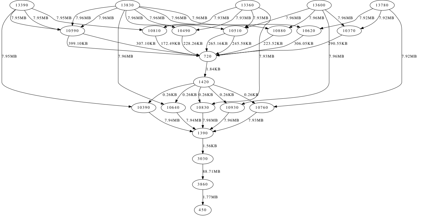
Figure 7: The Montage workflow with 25 nodes. The labels on edges represent volume of communication; The labels on vertexes represent computational time.
