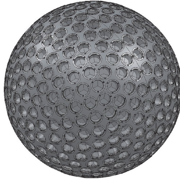
Fig. 2. LARASE model of the LAGEOS II satellite. LAGEOS II is one of the best tracked satellites all over the world by the SLR technique. LAGEOS II is almost twin of the older LAGEOS. The satellites structure is constituted by two hemispheres of aluminum containing 426 cube corner retroreflectors (CCRs), a brass core that contributes to increase the mass of the satellites and a Copper-Beryllium shaft that allows to fasten the different parts of the satellites. The heavy brass core was necessary to guarantee a low area-to-mass ratio for the two satellites, about 6.95 \times 10^{-4} \text{ m}^2/\text{kg} , the smallest among the laser-ranged satellites till the recent launch of LARES. LAGEOS II orbit has an inclination of about 53^\circ over the Earth's equator, a semi-major axis of about 12,163 km and an eccentricity of about 0.014. LAGEOS has an orbit inclination of about 110^\circ , a semi-major axis of about 12,270 km and an eccentricity of about 0.004. The smaller inclination of LAGEOS II has been chosen to obtain a better visibility from the network of the Earth laser ranging stations.
