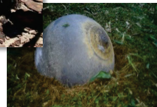
Spherical tank from the 2 nd stage of Zenit 3F, found in the Tuyen Quans Province, Vietnam (2016)
