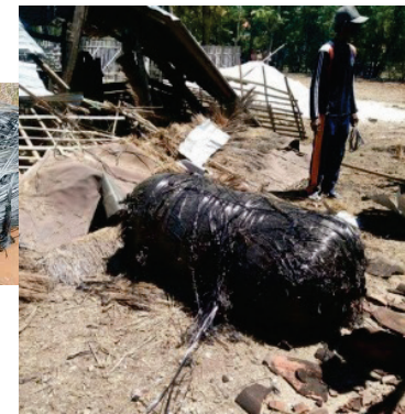
Pressure vessel from the 2 nd stage of Falcon 9, found on the island of Giliraja, Indonesia (2016)
