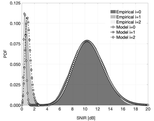
Fig. 2: Example of empirical PDF vs. SNIR model ( $G = 0.5$ ,  $i = \{0, 1, 2\}$ ).
