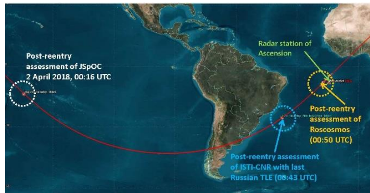
Fig. 25. Post-re-entry estimates (at the geodetic height of 10 km) by Roscosmos and ISTI-CNR, based on the latest Russian TLE, compared with that of JSpOC, based on the latest American TLE.
