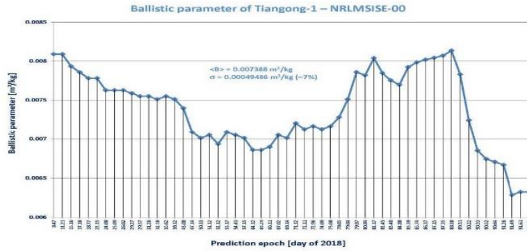
Fig. 16. Evolution of the Tiangong-1 ballistic parameter determined at ISTI-CNR with the density model NRLMSISE-00.
