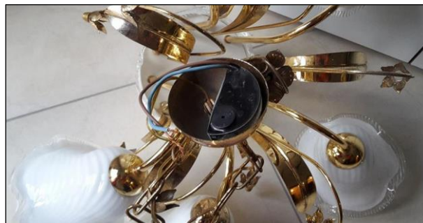
Figure 3: Prototype placed in the ceiling support of the chandelier
