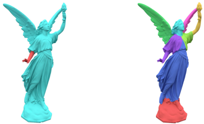
Figure 9: Segmentation of the Lucy model with different dimensions for the printed object, using the same parameter t = 3mm . For the smaller Lucy (left), few pieces are preferred. More pieces are allowed for the bigger Lucy (right), as the pieces would be easier to 3D print and assemble.
