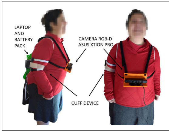
Fig. 2: The proposed navigation system worn by the user. We can see the wearable technological device, the camera and the processing unit (laptop): front view on the right, lateral view on the left.
