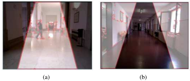
Fig. 3: In these pictures it is possible to observe an example of the analysis of the corners inside the three subareas of investigation: central area (a), and lateral ones (b).
