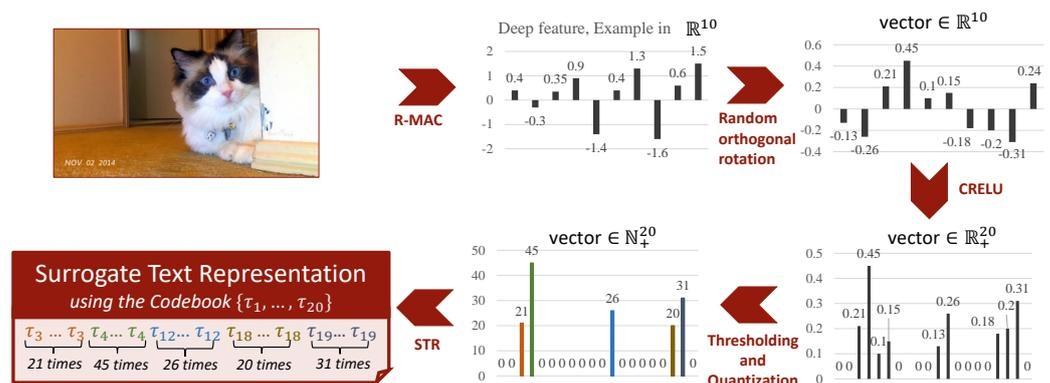
**Figure 8.** Scalar Quantization-based Surrogate Text representation: clockwise the transformation of the image R-MAC descriptor- depicted as a 10-dimensional vector- into a textual encoding called Surrogate Text Representation.
