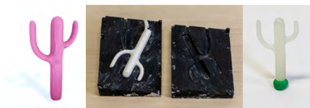
Fig. 10. For a simple object, our method can derive a single two-piece rigid mold as in [Stein et al. 2019].
