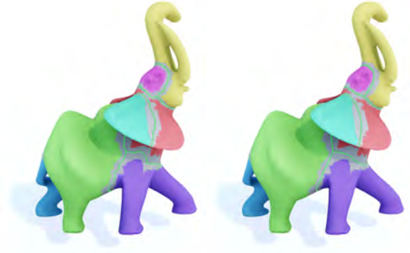
Fig. 6. Boundary seams smoothing. Left: the surface seams polyline (green), derived from the DHF partitioning, can freely move within a tolerance region (gray) while preserving DHF-accessibility of the surface regions it delimits. Right: the same polyline is smoothed using the tolerance region as smoothing domain.
