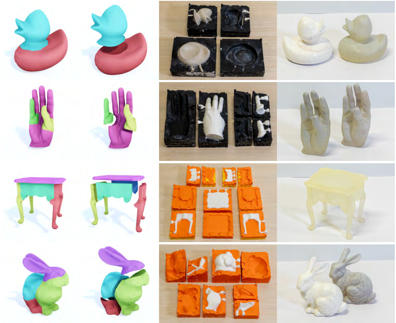
Fig. 11. Segmentation and fabrication result: for each model we show the tetrahedral decomposition, the final DHF parts, the fabricated molds with their respective cast part, and the final assembled results.
