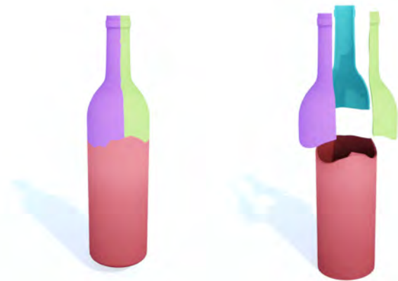
Fig. 12. A model with a complex occlusion configuration, like a bottle, can be successfully automatically decomposed and fabricated with the proposed method.
