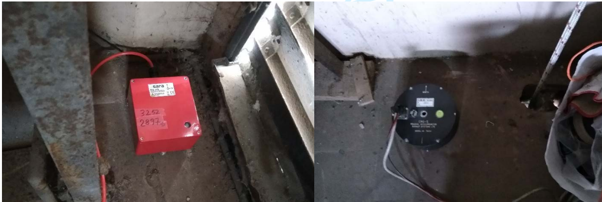
Figure 6. A seismic station (on the left) and an accelerometer installed on the bell tower.
