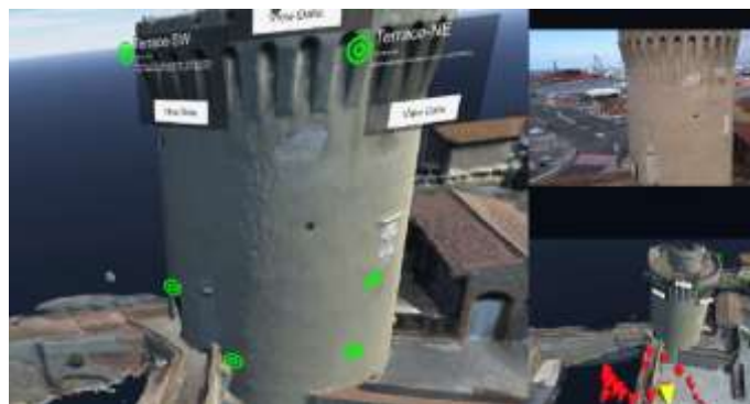
Fig. 4 – The VR interface is composed of three elements: (i) the central part shows a reconstructed virtual scene with installed sensors and their gathered values; (ii) on the upper right side of the screen, the video recorded by the UAV during the inspection operations is shown; (iii) in the lower right side, a panoramic view of the virtual scene is displayed reporting also UAV actual position (yellow pyramid) and travelled path (represented as a set of smaller red pyramids). Please, see http://moscardo.isti.cnr.it/ for an interactive demo.
