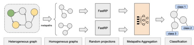
Figure 13. Pipeline proposed in [61] to process knowledge graphs to classifying the nodes given the node attributes and the node neighbourhood.
